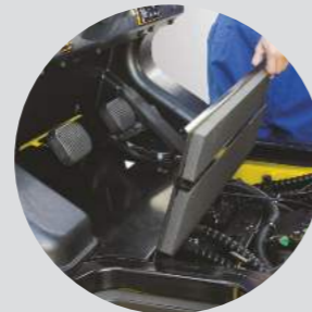
One Touch, No Tool Floor Plate
